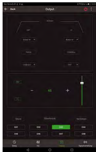
The crossovers can also be set with the app, as well as runtime, level etc.
