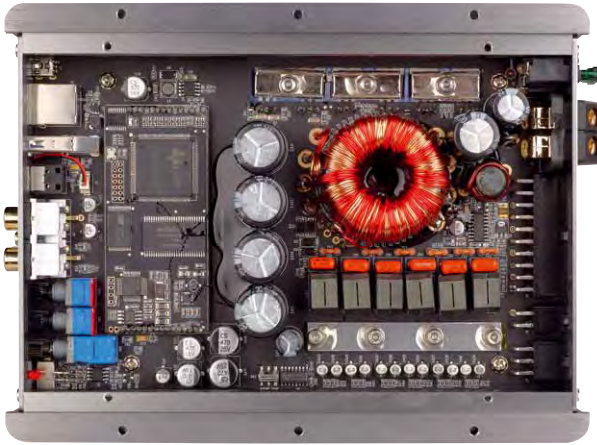
The 6 channels are amplified with 3 chips. The DSP sits with controller and memory on an additional board
