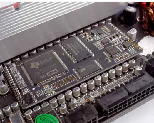
The DSP board contains the large TI DSP, the controller and two memory chips
