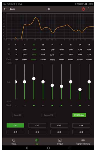
The app offers almost full functionality, here with equalizers and frequency response
