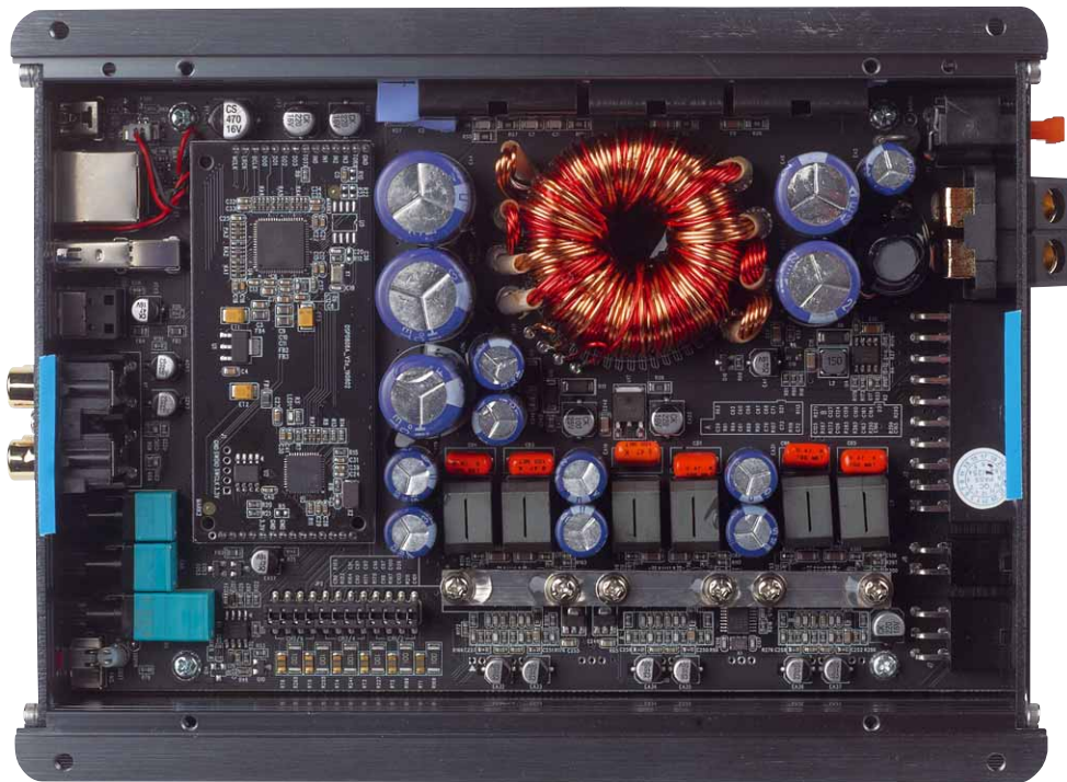
Located on the left of the daughterboard DSP. The jumper for switching between high and low is located at the bottom
